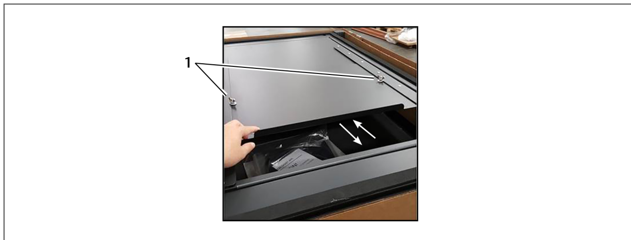
Figure 4.27 Adjusting the air-flow dampers
